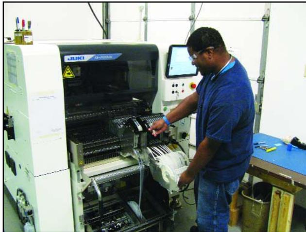
*Jarrell Paxton, MSI electronics assembler, loads reels into the KE-3020.*
